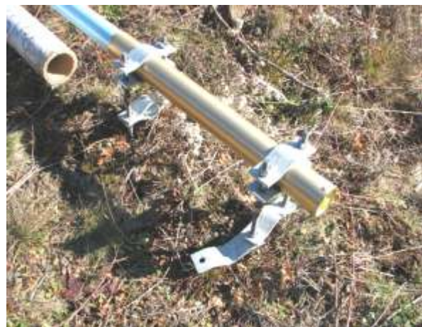
Look at the brand new Telewave 6 dbd 22' tall Fiberglass antenna with its gold anodized mounting base
